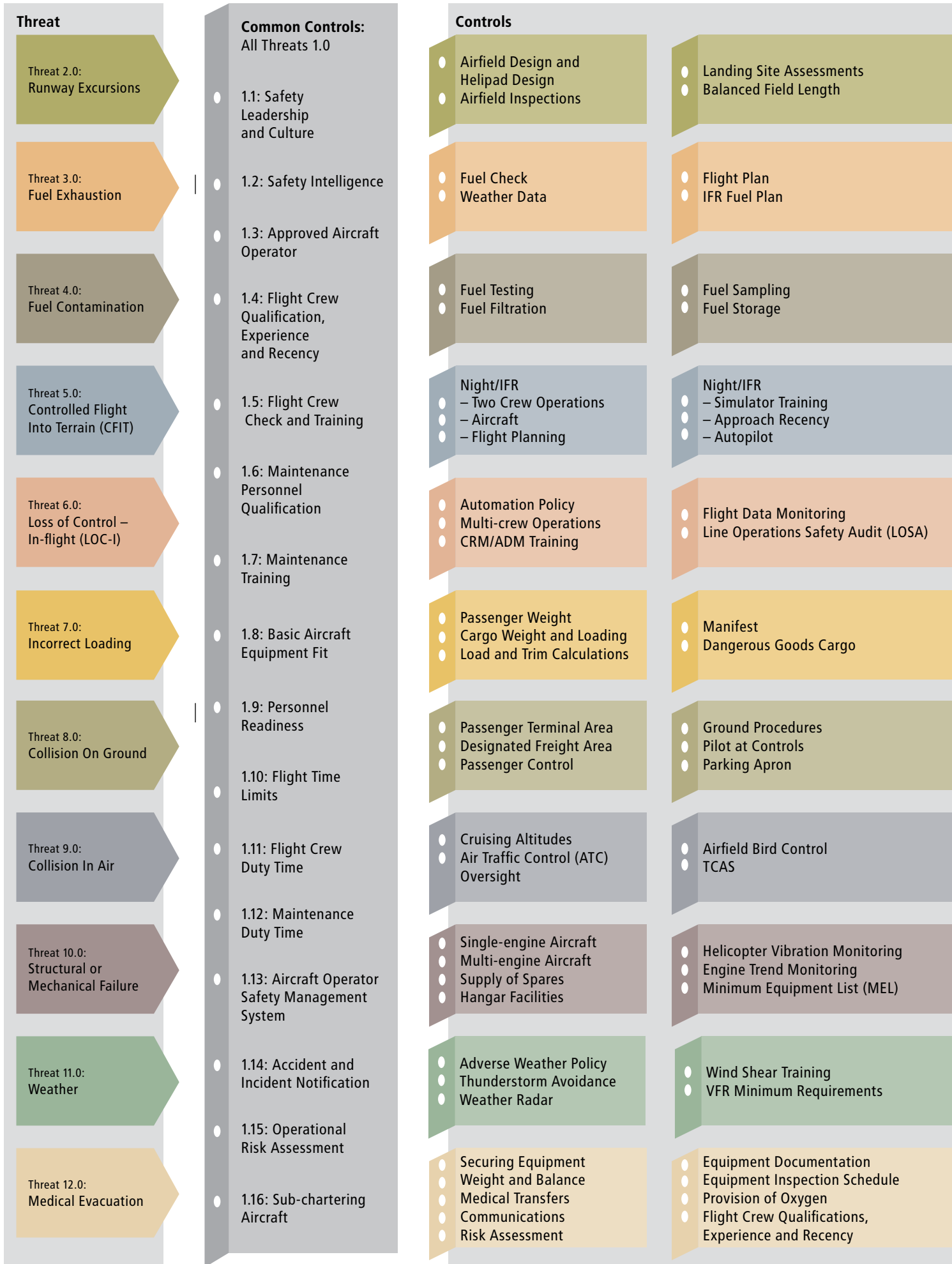
Figure 1: BARS Bow Tie Risk Model – Schematic of Aviation Risk Management Controls and
